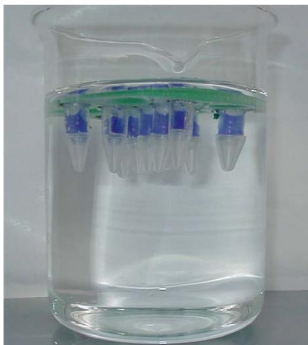
**Figure 3:** Dialysis with Mini *GeBAflex-tube*.
