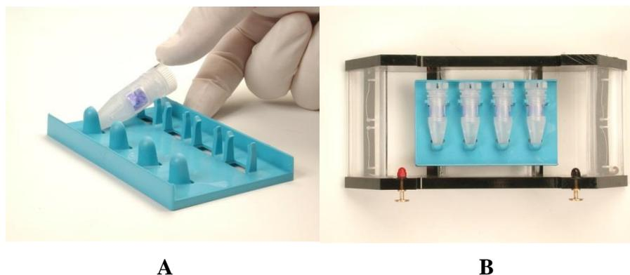
**Figure 1:** (A) Insertion of Midi GeBaFlex-tube in Midi Supporting Tray showing correct orientation of membranes, which must be perpendicular to the electric field. (B) Supporting Tray containing four GeBaFlex-tubes in a horizontal electrophoresis tank. Membranes of each tube are perpendicular to the electric field.
