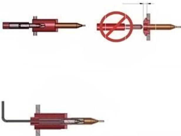
4. Make sure that the adapter is locked into the socket.
